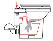
When the flush handle is pressed the flapper opens, allowing wastewaterto flow into the hopper. Clean water enters the bowl from the rim to thoroughly wash the bowl.
