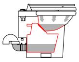
After 4-8 seconds, the flapper closes. Cleanwater continues to flow into the bowl,where is remains until the next flush.
