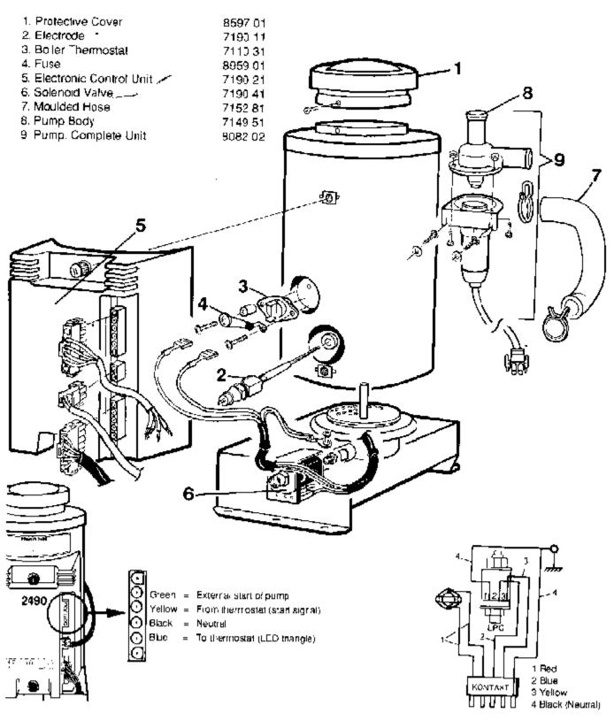
When replacing the solenoid valve leave the beiter in original position, unscrew the gas pipe, disconnect electronic control unit and remove the two screws that hold it in position. The unit can then be removed from the front of the boiler.
