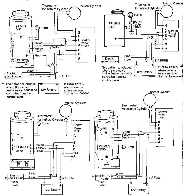
For model 2470 boiler with electric in-line heater and indirect cylinder
