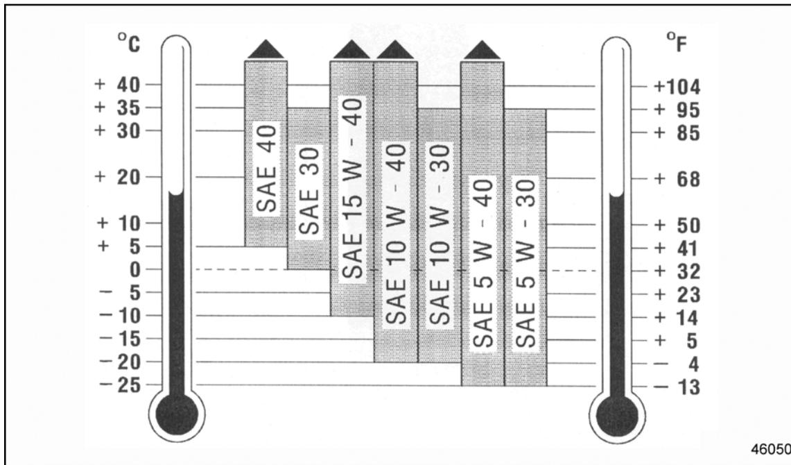
**Figure 3-1** Temperature Limits for Oil Viscosity Grades
