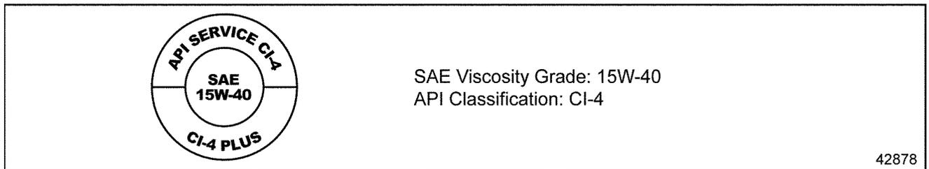
Figure 2-1 API Symbol: 4-Stroke Cycle Engine Oils
