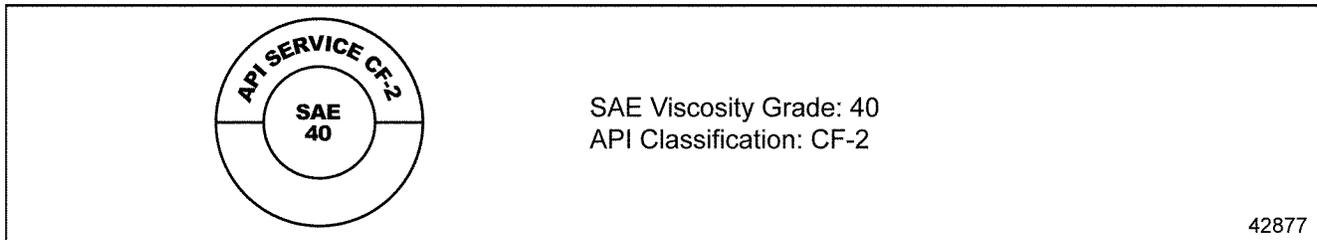
**Figure 2-2 API Symbol: 2-Stroke Cycle Engine Oils**
