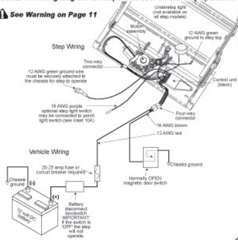
**FIGURE 12: Wiring diagram for steps without control unit**
