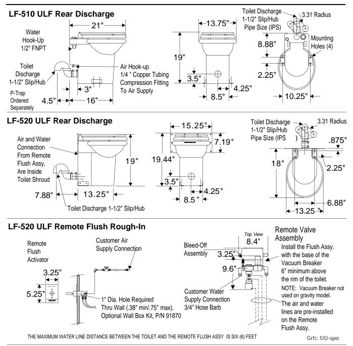
**TOILET SEAT:** Toilet seat post holes are on standard 5-1/2" centers. The seat is provided with most units. **DOWNWARD DISCHARGE KIT:** An optional Bottom Discharge Kit, P/N 93702, can be ordered to convert rear discharge models to downward discharge. Contact factory for details.
