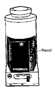
The system's heat source is the model 2480 boiler, which has an output of 3 x 2.1 kW, giving a maximum output of 6.3 kW. Two of the three burners are operated by solenoid valves. The third ourner is operated manually.
